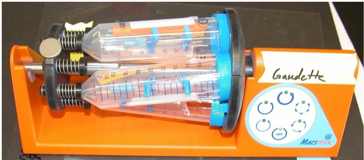
Figure 6: Microthreads placed in tube rotator
